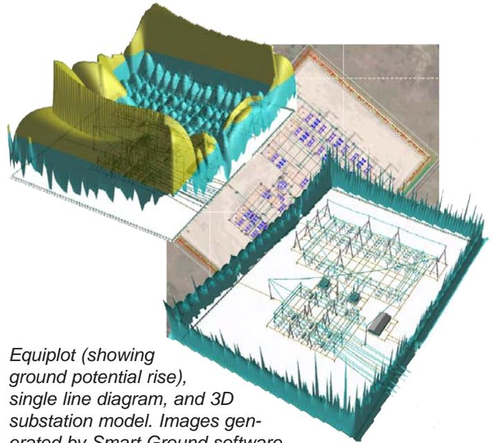
*Equiplot (showing ground potential rise), single line diagram, and 3D substation model. Images generated by Smart Ground software.*
